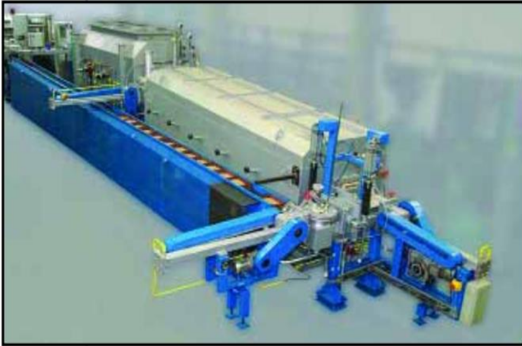
Fig.I.12: PM Continuous sintering furnace, courtesy of Elinofurnaces GmbH [21].
