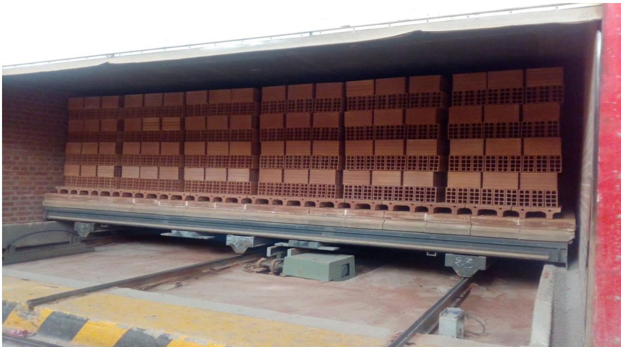
Fig.III.5: The output of bricks product from the furnace.
