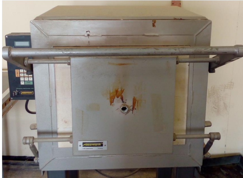
Fig.III.15: Sintering furnace (Nabertherm).
