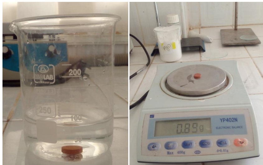
Fig.III.16: Water absorption test (immersion).
