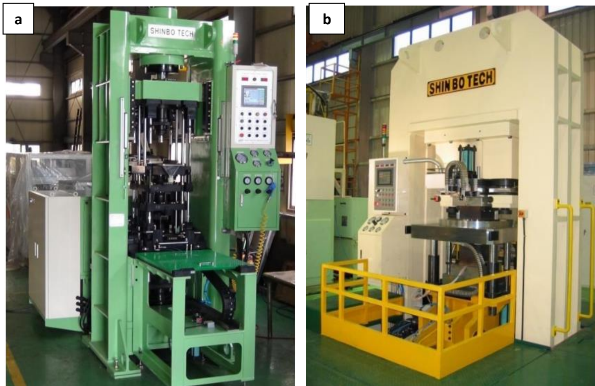
Fig.I.5: Hydraulic auto powder compacting press; a) cold press ranging from 30 tons to 500 tons, b) Hot press with mold heating systems (400°C), ranging from 30 tons to 2000 tons [12].
