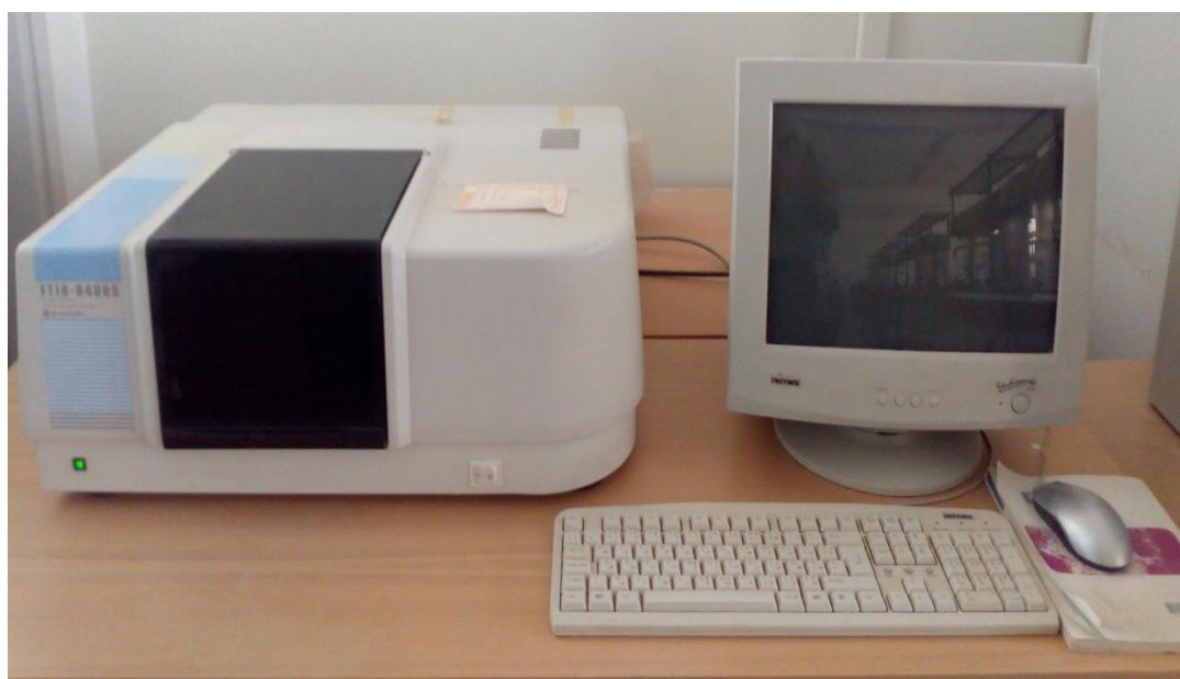
Fig.III.11: Machine of infrared spectroscopy analysis (FTIR 8400S).
