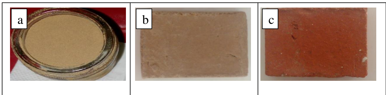
Fig.III.7: Samples from SARL Eloutaya. Poterie; a) mixture of powders before molding, b) dried sample at 80°C, c) sintered sample at 850°C
