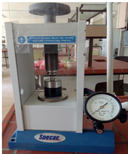
Fig.III.14: Compacting press (Specac).
