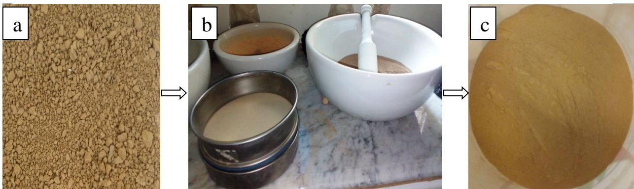
Fig.III.9: Milling and sieving operations in laboratory:a) coarse clay, b) milling and sieving, c) fine clay(grain size less than 315 \mu m).
