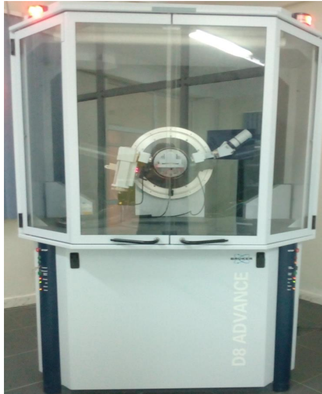
Fig.III.12: Bruker D8 advance machine.
