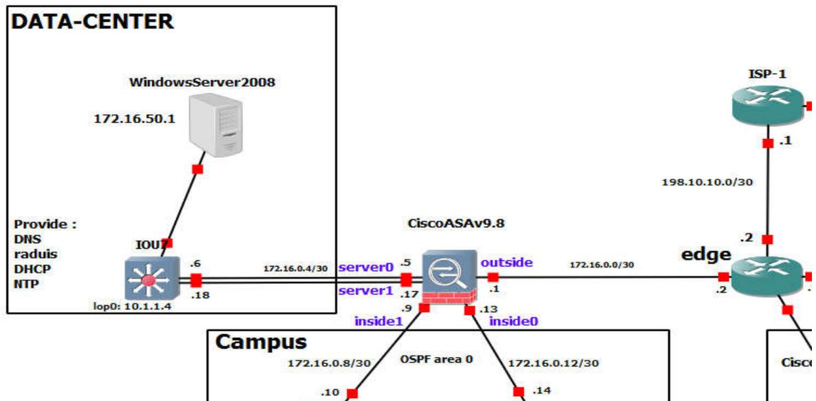
**Figure 3.4 :** CiscoASA9.8, Campus, DATA-CENTRE and edge Connection.
