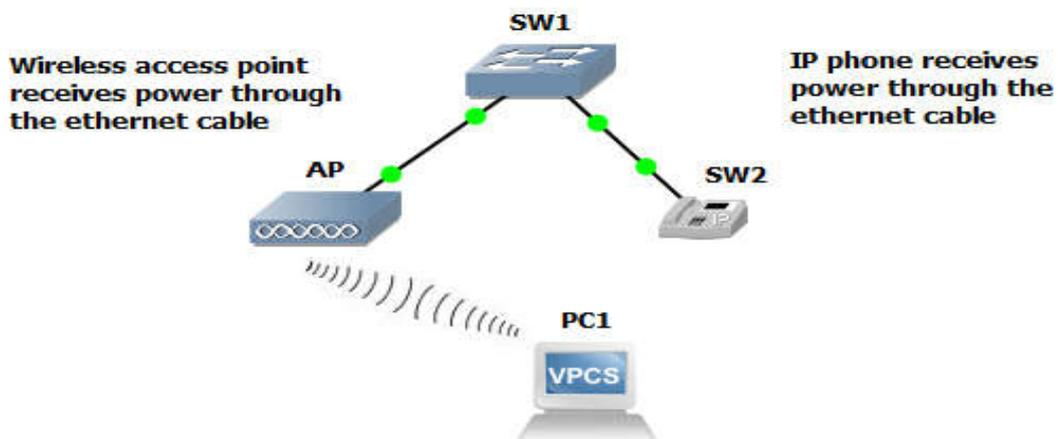
**Figure 1.11 :** Power over Ethernet.
