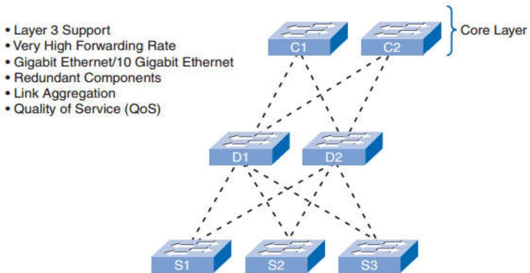
**Figure 1.14 :** Core Layer Switch Features.
