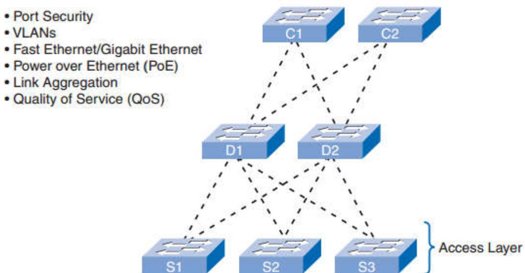
**Figure 1.12 :** Access Layer Switch Features.
