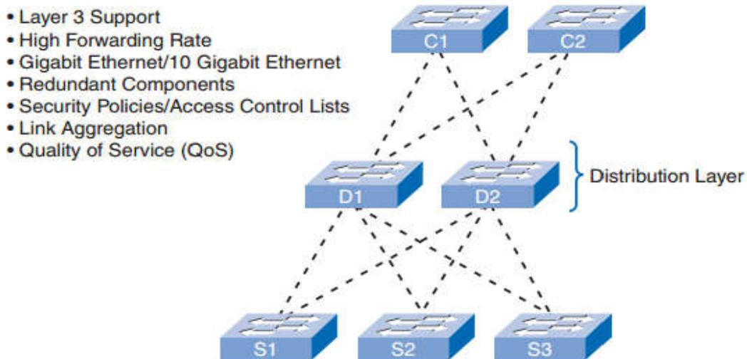
**Figure 1.13 :** Distribution Layer Switch Features.
