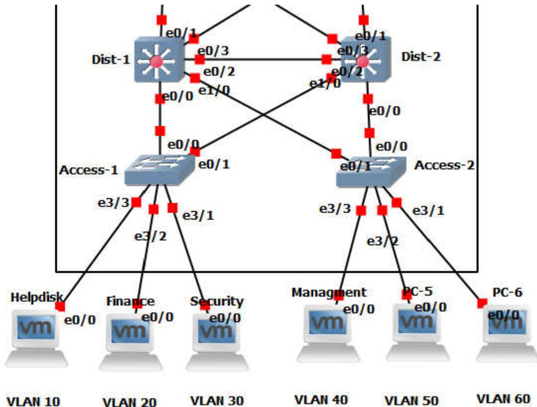
**Figure 3.2 :** Access Switches Connected to Distribution Layer.
