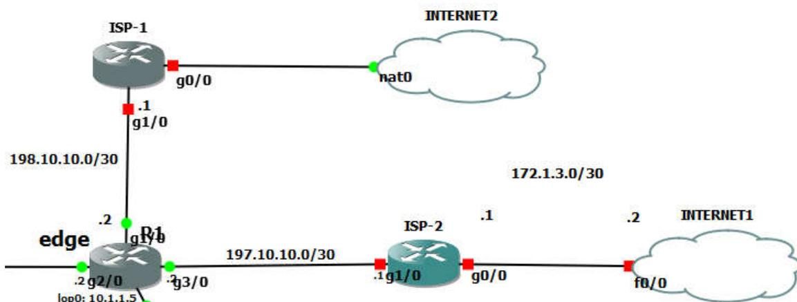
Figure 3.7 : Company Connection to the Internet via edge router.
