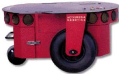
Figure II.6 Le Robot mobile Pioneer P3-DX [13].
