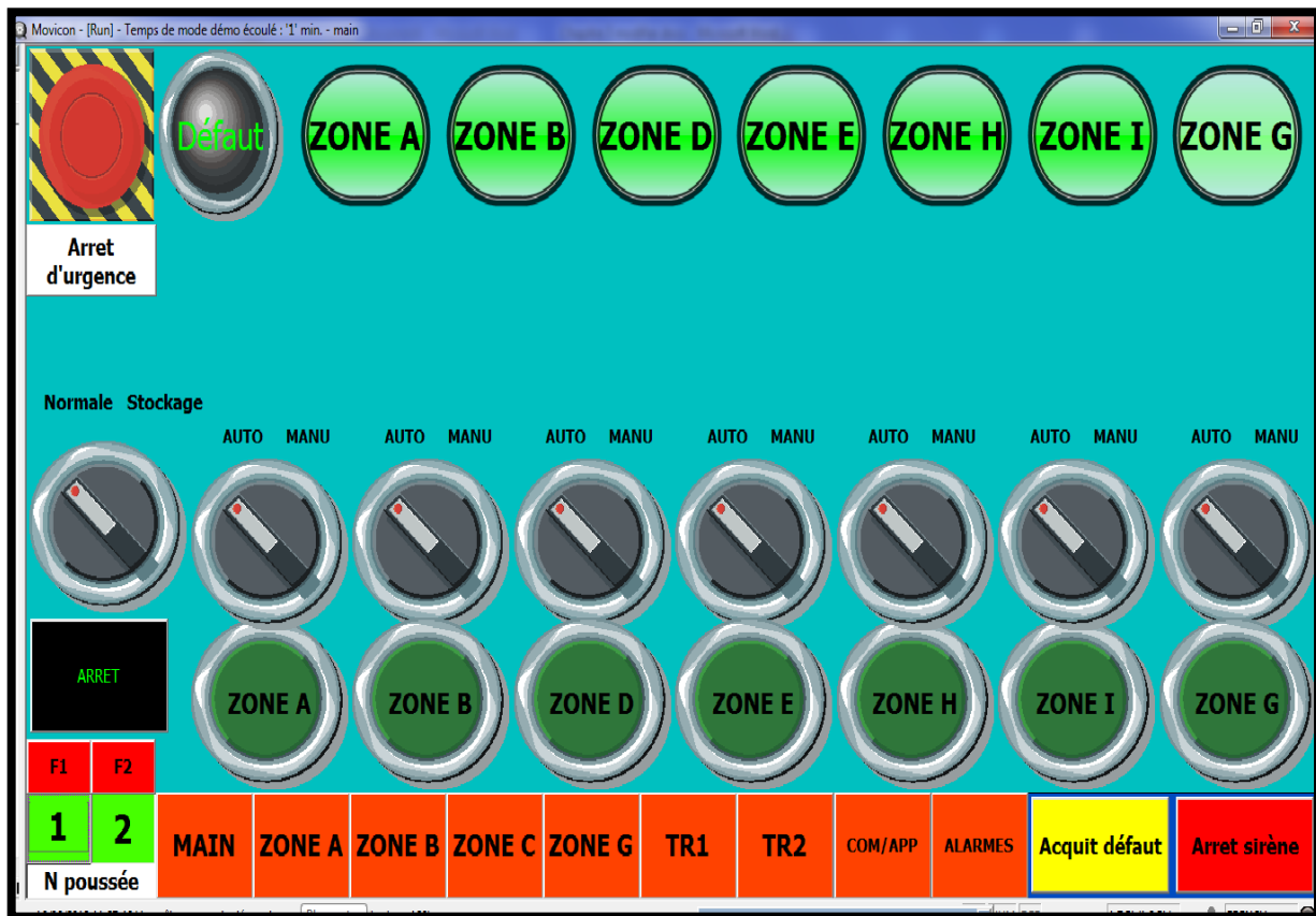
Figure III.8 : Synoptique MAIN (principale)
