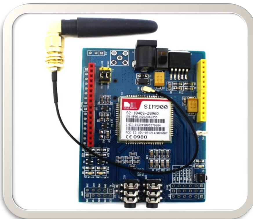
Figure III.30: Carte Sim 900 GSM/GPRS shield.
