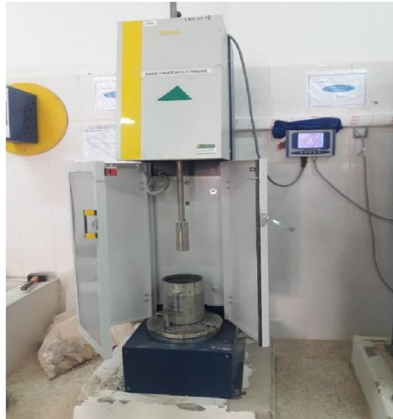
figure IX-7-Appareille de proctor
