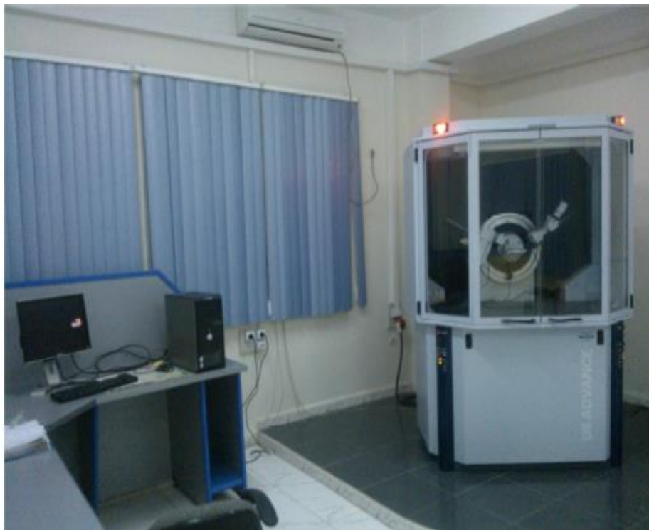
Figure III.3: Diffractomètre Panalytical X'pert (D8 ADVANCE) BRUKER.
