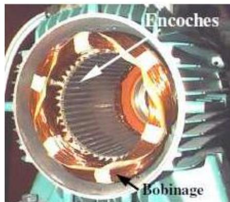
**Fig. I.2 :** Stator de la machine asynchrone.
