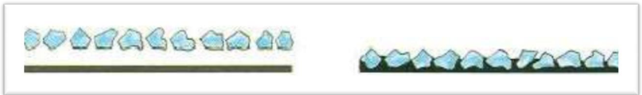
Figure III.2 : Structure monocouche simple gravillonnage
