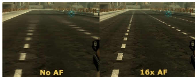
FIGURE 2.16: The huge difference between with and without Anisotropic filter as the distance goes higher. Source: [44]
