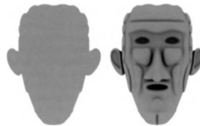
(B) Ambient Occlusion versus a constant ambient term. Source: PRT-Demo, Microsoft SDK, November 2007
