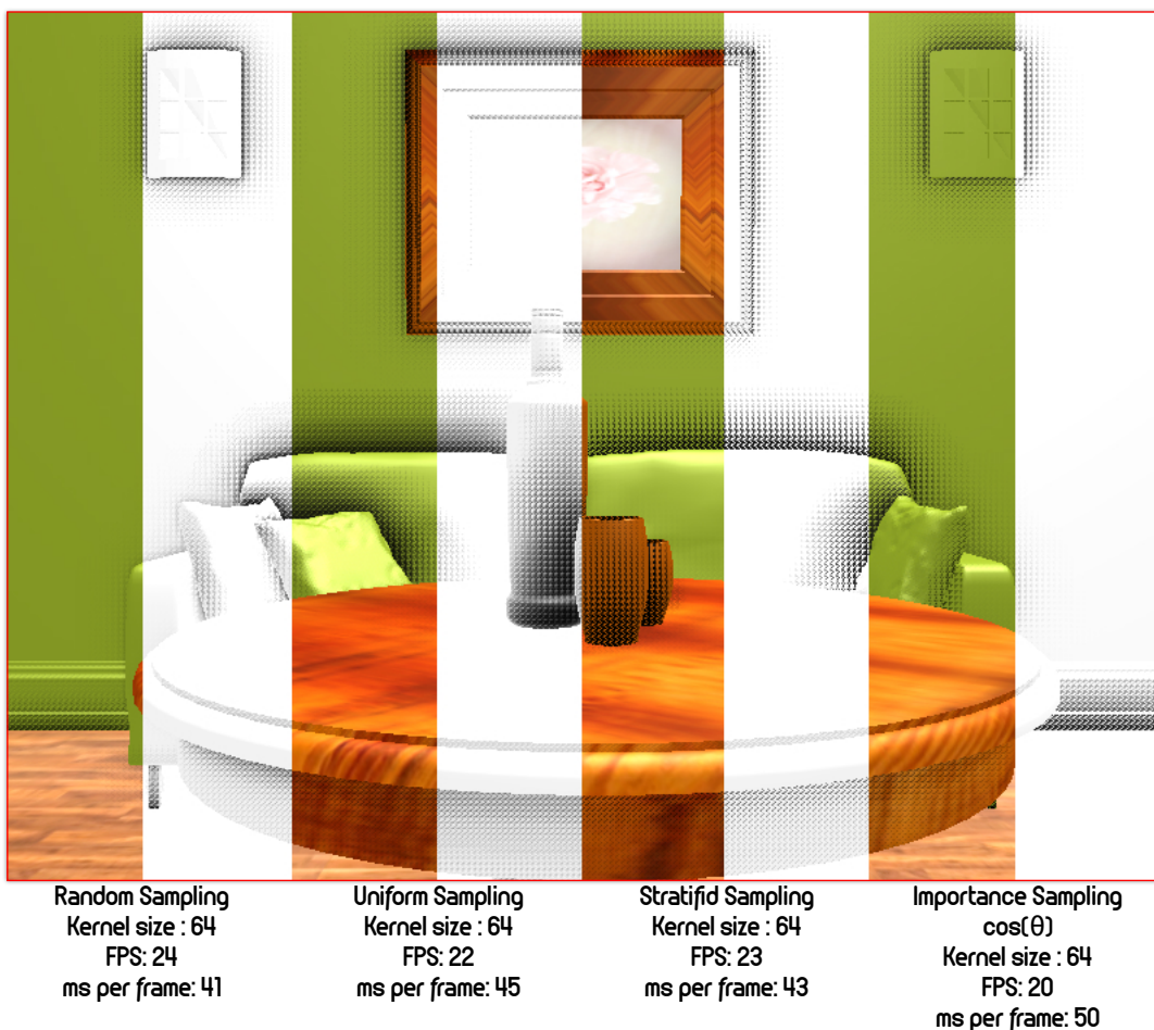
FIGURE 4.11: AlchemySSAO factor calculated using random, uniform, stratified, importance sampling techniques.
