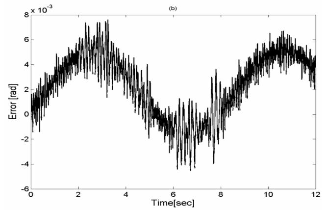
Figure 12: Tracking performances and control activities of PD controller in disturbed case.
