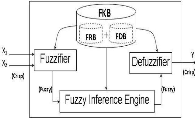
Figure 1: Structure of the fuzzy logic control.
