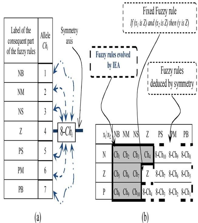
Figure 3: (a) Symmetry mechanism of labels in the consequent part of fuzzy rules, (b) FRB parameters to be evolved by IEA.
