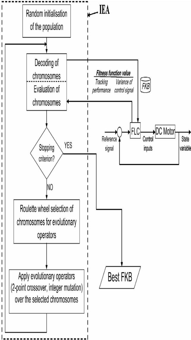
Figure 4: Integer evolutionary fuzzy control system configuration
