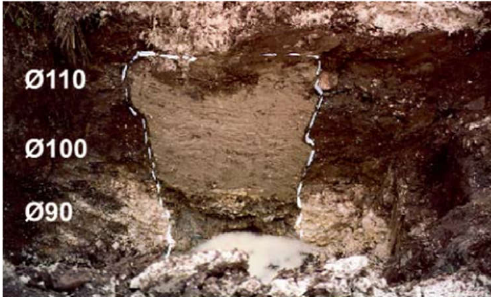
Figure III .8 Jet simple (document Solétanche Bachy) .
