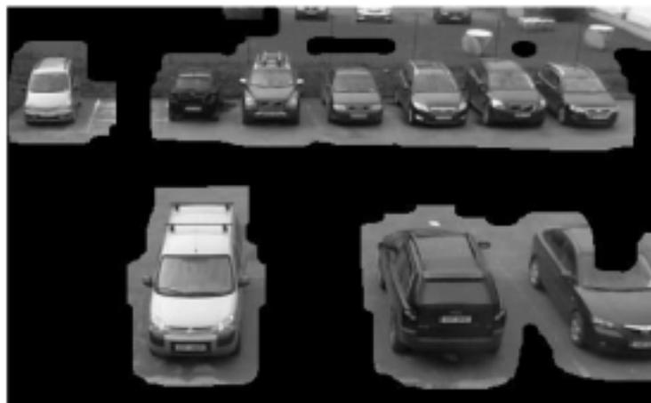
FIGURE 3.5: MOG with dilation and erosion.[24]
