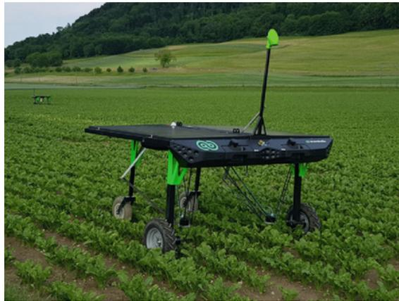
FIGURE 1.5: Autonomous mobile robot weeding a field [2]
