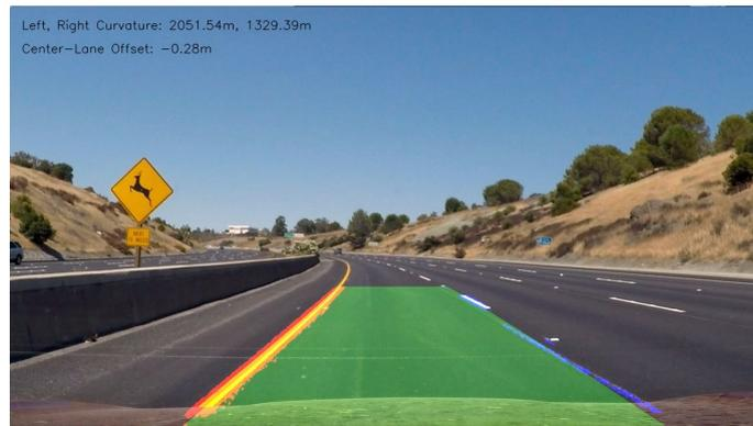
FIGURE 3.9: Tracing road by HSV method.
