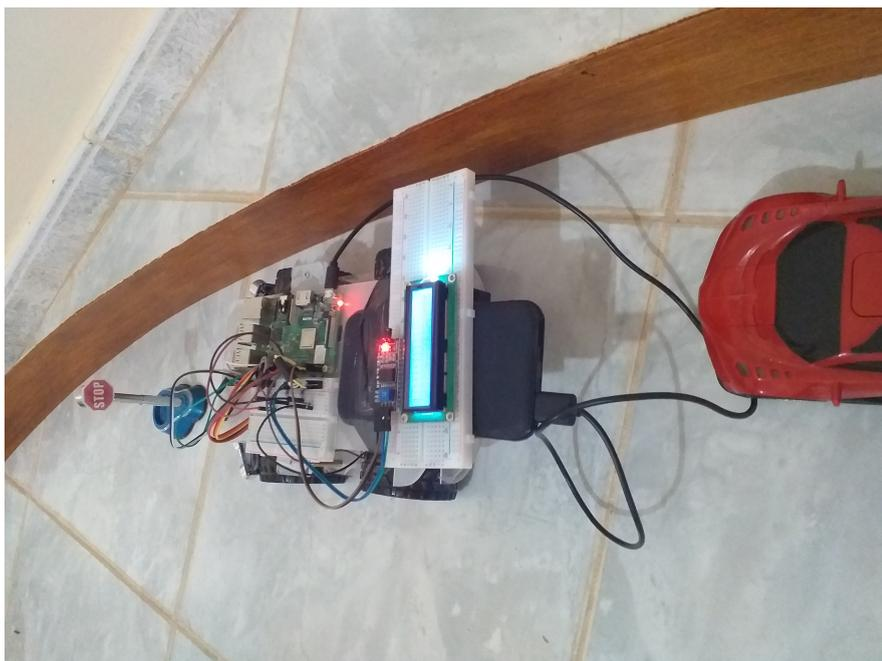
FIGURE 5.26: Autonomous car detect stop sign.
