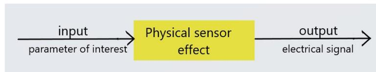
FIGURE 2.1: Principle of a sensor [14]
