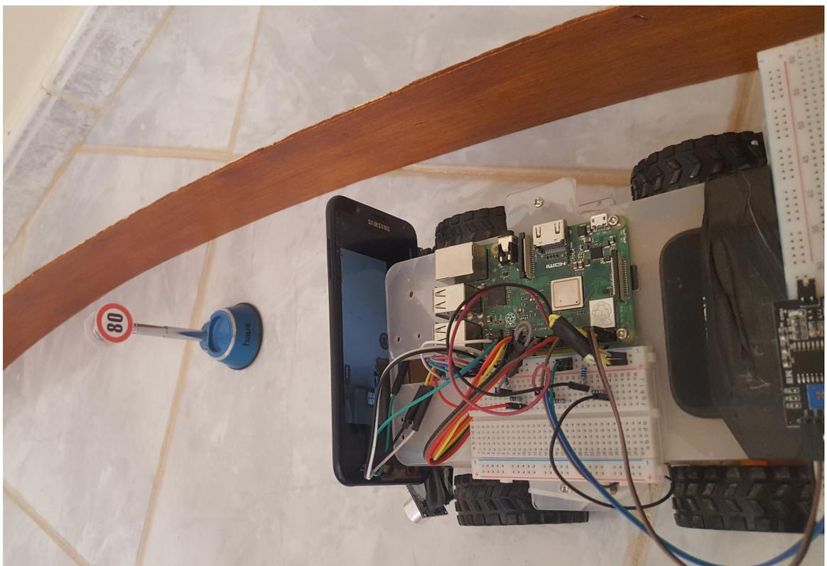
FIGURE 5.28: Autonomous car try detect sign Maximum speed 80 km/h.
