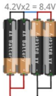
Figure 14 batteries joined in series and parallel
