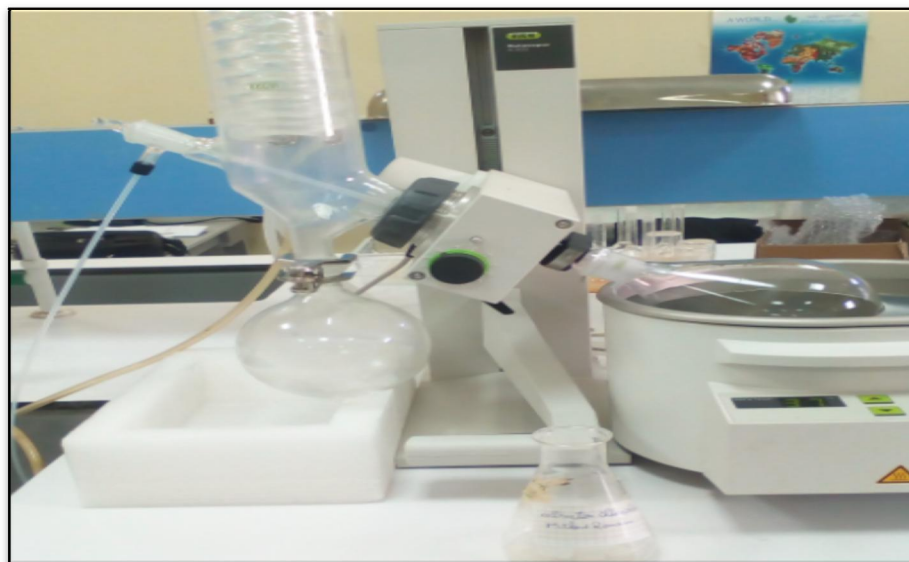
Figure .14 Evaporation rotative (Rotavapor)
