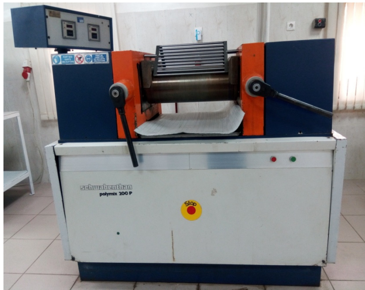
Figure .III.5 : calandre de type schwabenthanpolymix 200p
