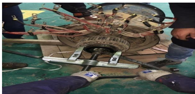
Figure III.44 Extraction du roulement.
