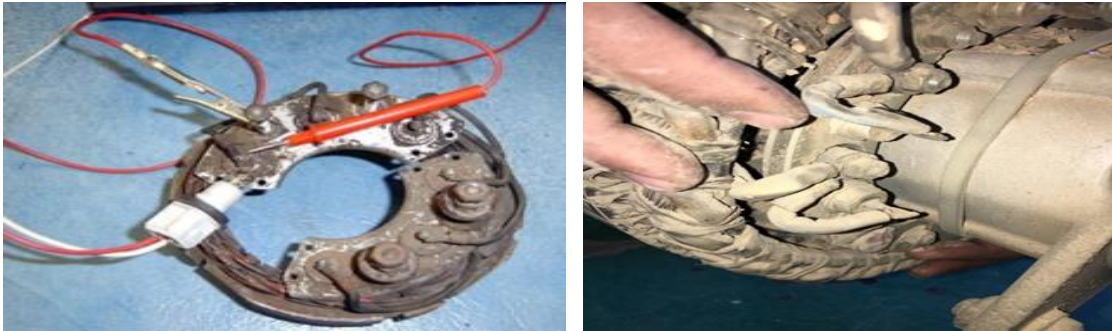
Figure III.39 Essai des diodes.
