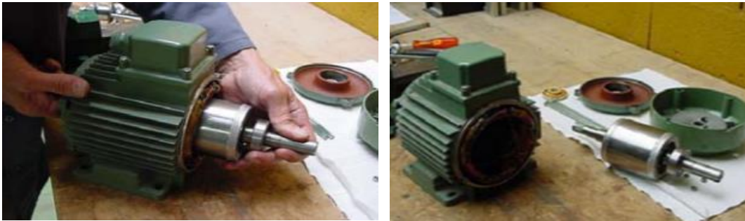
Figure III.14 Extraction du rotor. [15]
