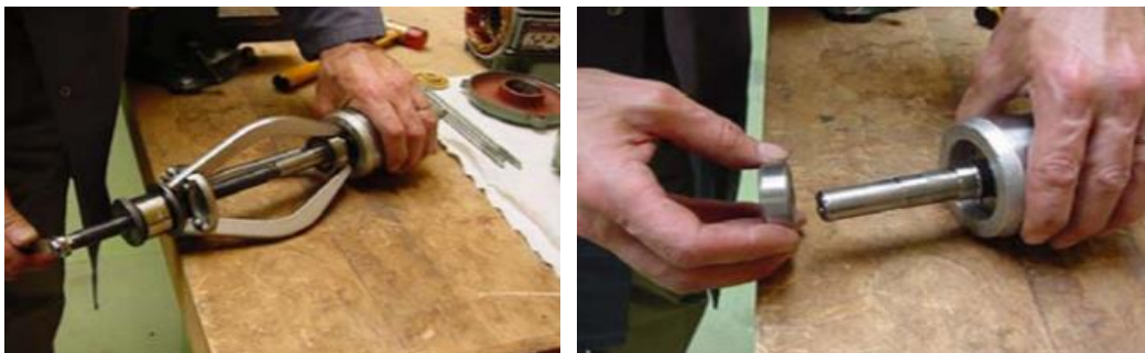
Figure III.16 Extraction du roulement. [15]
