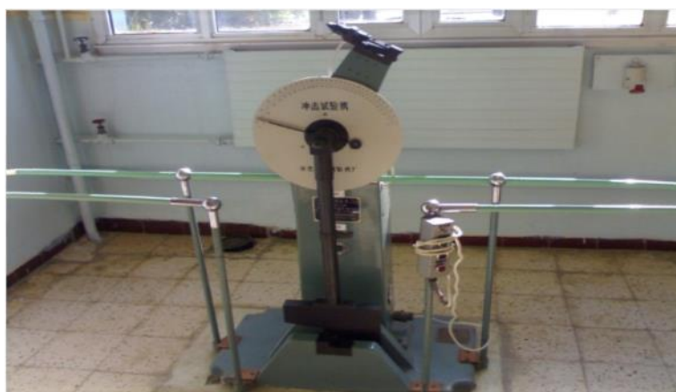
Figure III.12 machine d'essai de choc semi-auto
