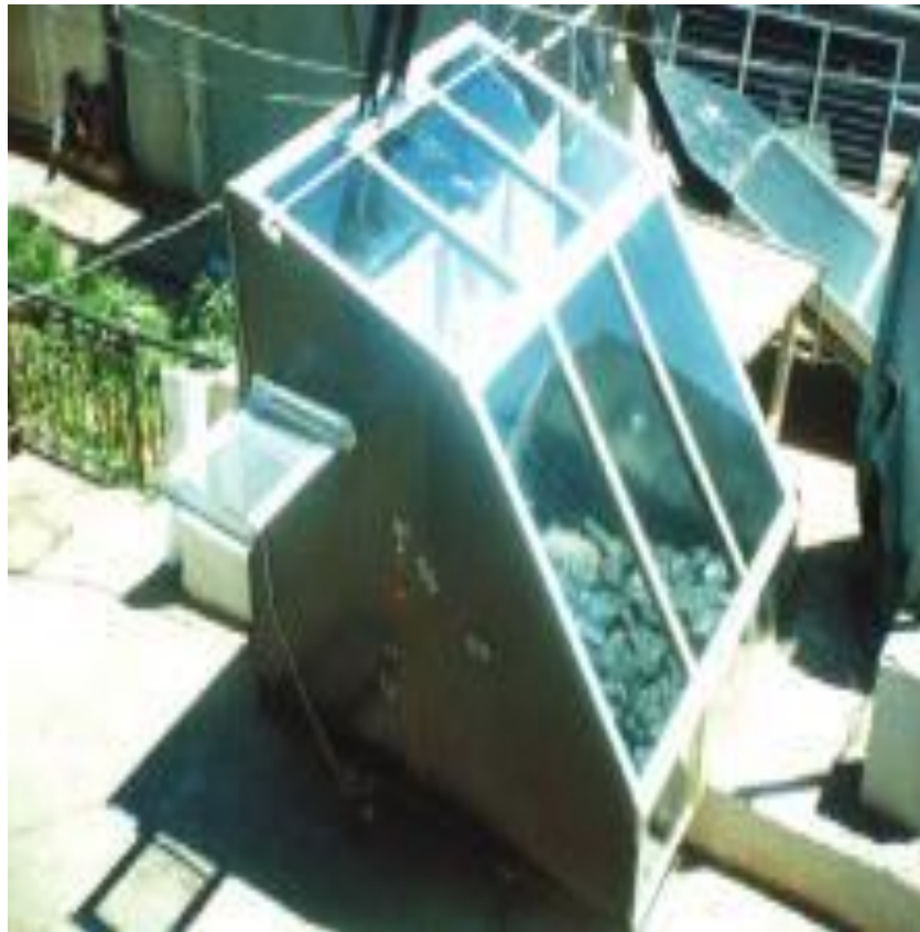
Fig.II.2 : Séchoir solaire direct. [5]
