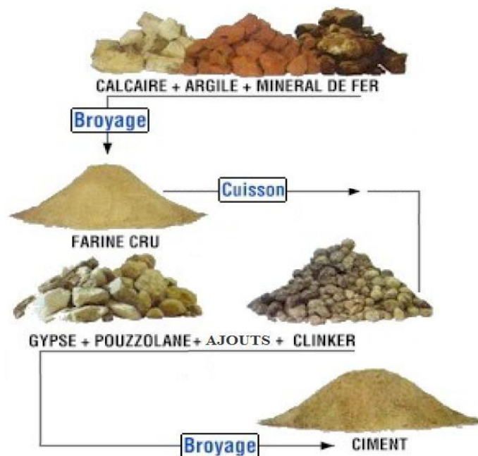
Figure 1: Cycle de fabrication de ciment [2]
