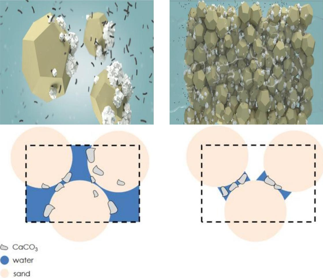
Figure 24: Schematic representation of *S. pasteurii* cells attaching on soil grains (Terzis and Laloui 2019)
