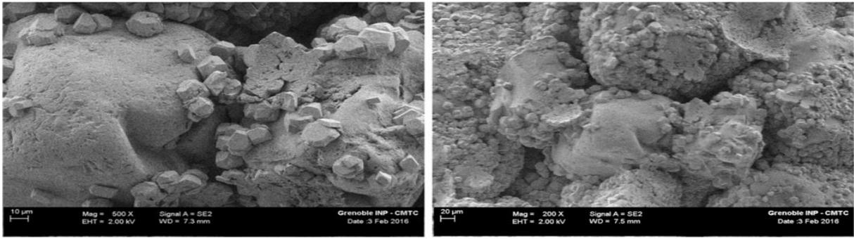
Figure 9: SEM observation of the biocemented sand by (Dadda et al. 2017)
