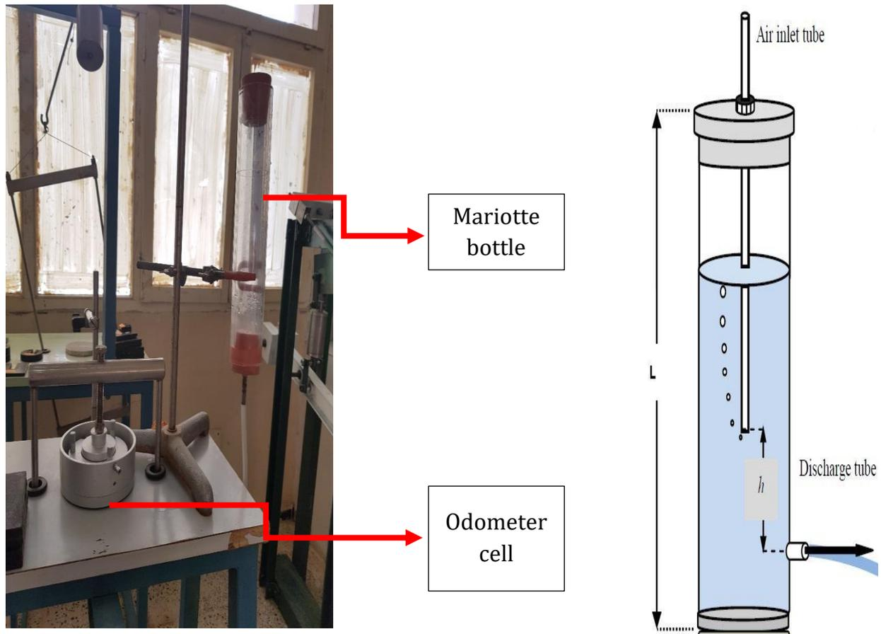
Figure 23: permeability measurement process
