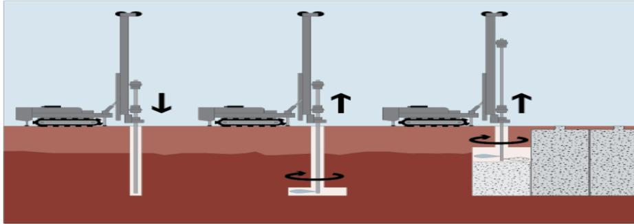
Figure 3: jet grouting
