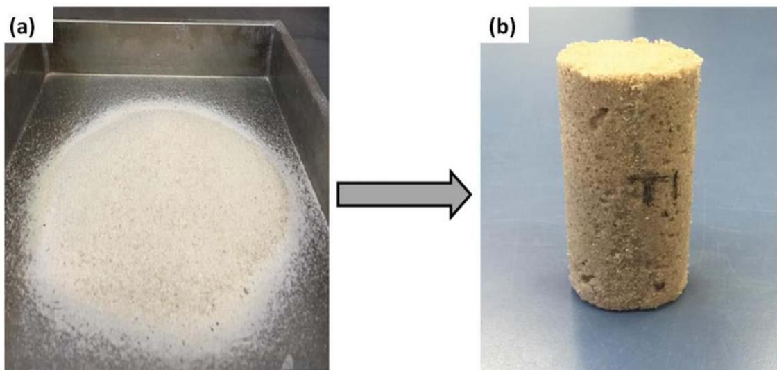
Figure 16. Sand metamorphosis: (a) natural sand; and (b) biocemented sand (bio sandstone) (Mujah et al. 2017)
