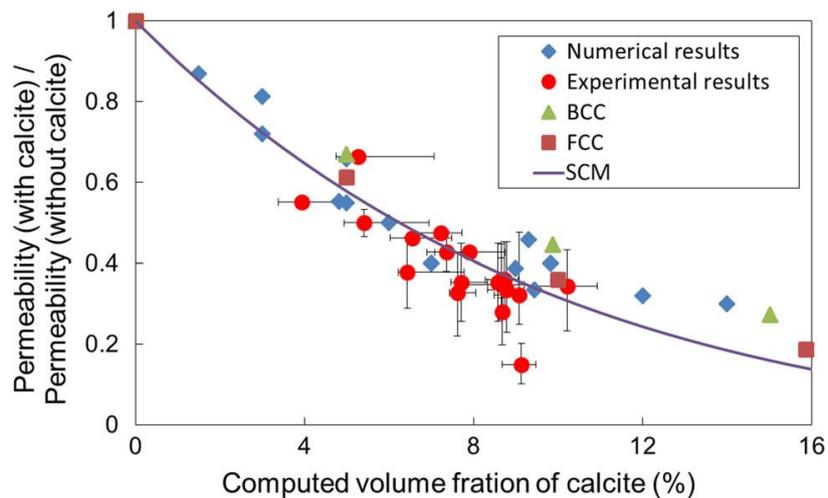
Figure 13. Evolution of the permeability ratio of the same sub-sample with and without calcite versus the volume fraction of calcite computed from 3D images (Dadda et al. 2017)
