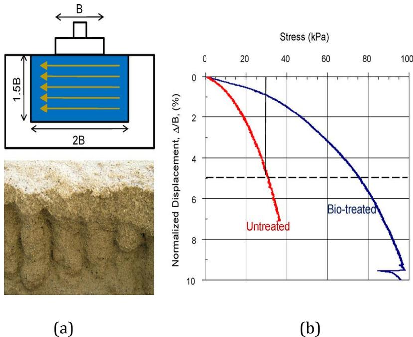
Figure 15. Experimental results from bio-mediated improvement of soil support a shallow footing foundation (DeJong et al. 2010)
