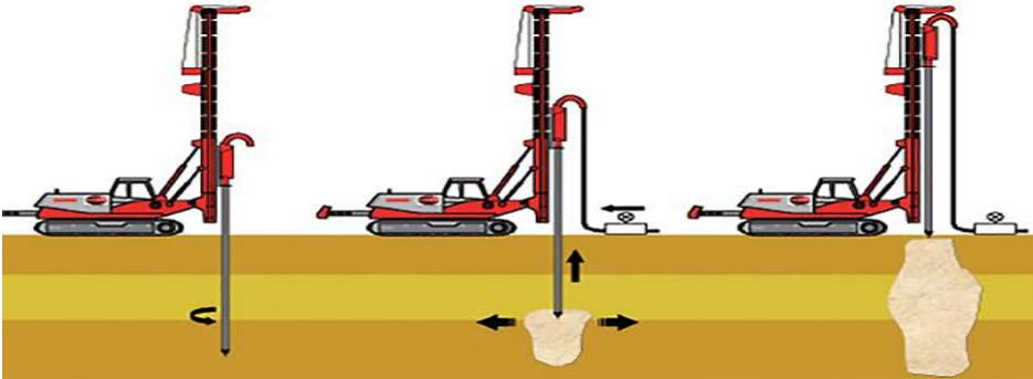
Figure2: compaction grouting
