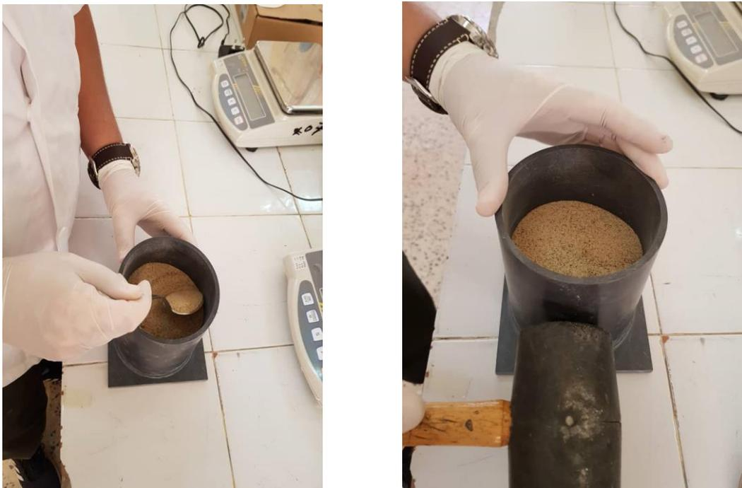
Figure 19: maximum voids ratio measurement
