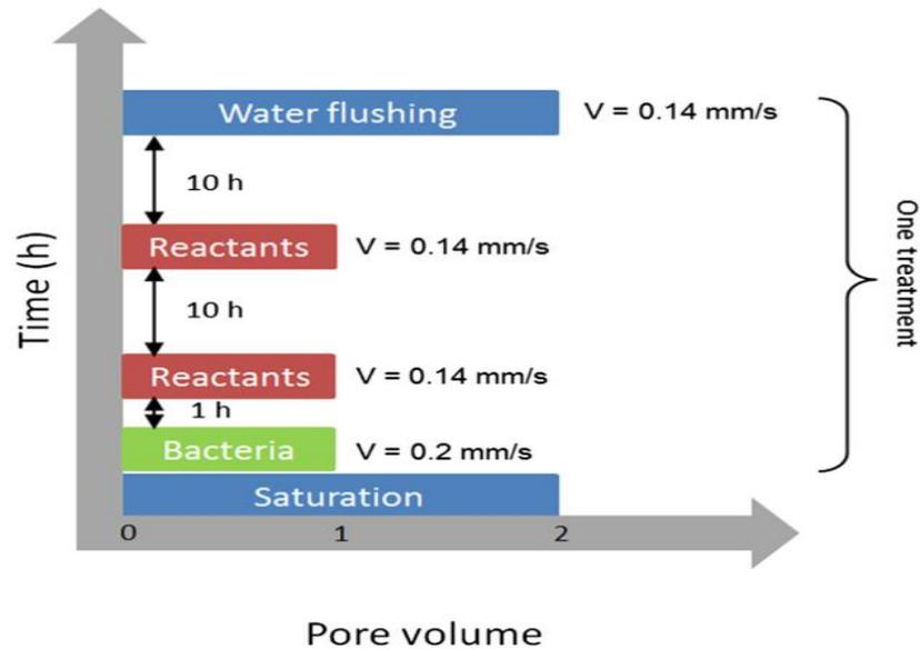
Figure 8: Injection protocol for biocementation process (Dadda et al. 2017)
