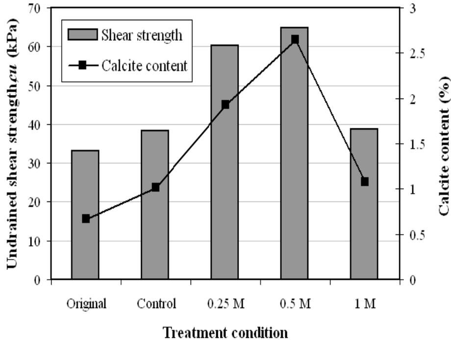
Figure 12. Shear strength and calcite content (Lee Min Lee et al .2012)
