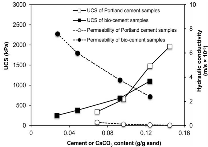
Figure 12: permeability of sand samples cemented with bio- cement CaCO<sub>3</sub> (100% saturation) and Portland cement (Cheng et al. 2013)
