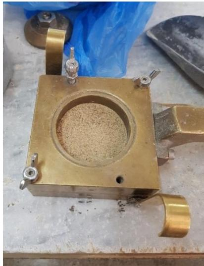
Figure 20: transfer sample into shear box
