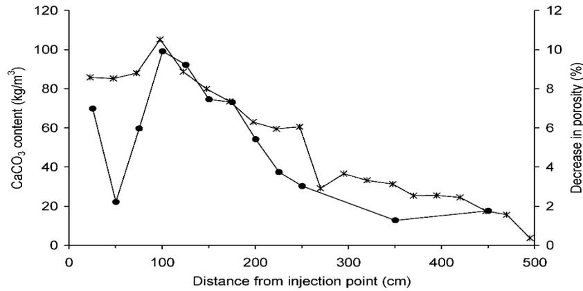
Figure 11: Relative decrease in porosity (•) versus calcium carbonate content (\*) over the length of the column by (Victoria S. Whiffin et al. 2007)
