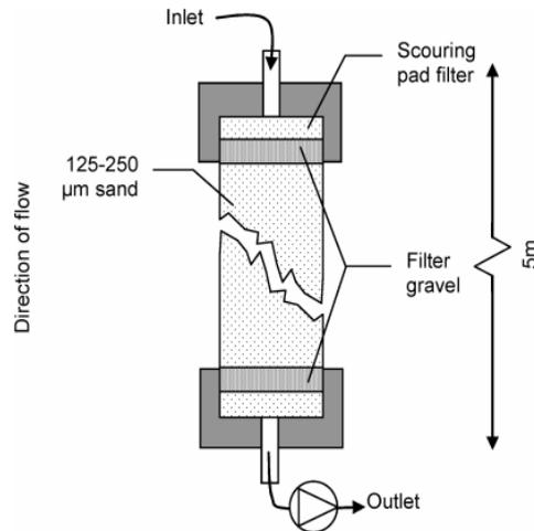
Figure 7: Schematic of column filter setup as (Whiffin et al.2007)
