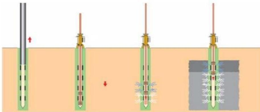
Figure 4: Diagram Showing Permeation Grouting
