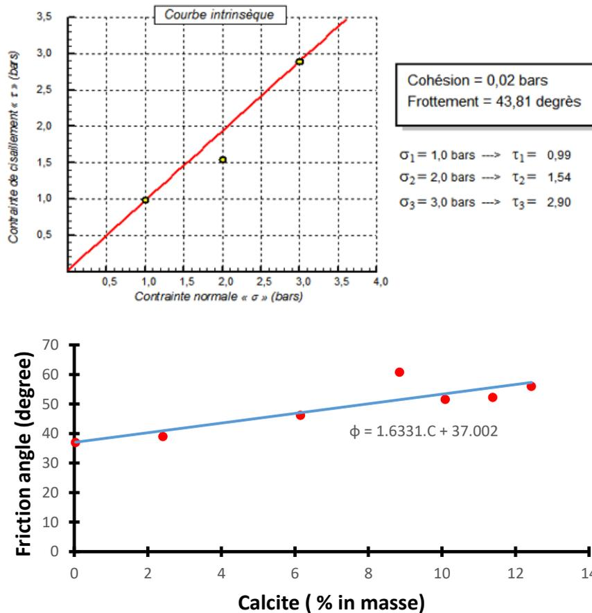
Figure 25: shear strength improvement: untreated (up), treated (down)
