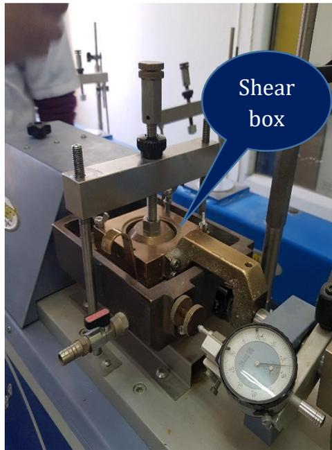
Figure 21: position of shear box
