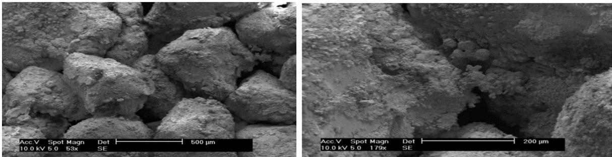
Fig. 10: Formation of  $\text{CaCO}_3$  crystals for samples treated at 100% saturation (Cheng et al. 2013)
