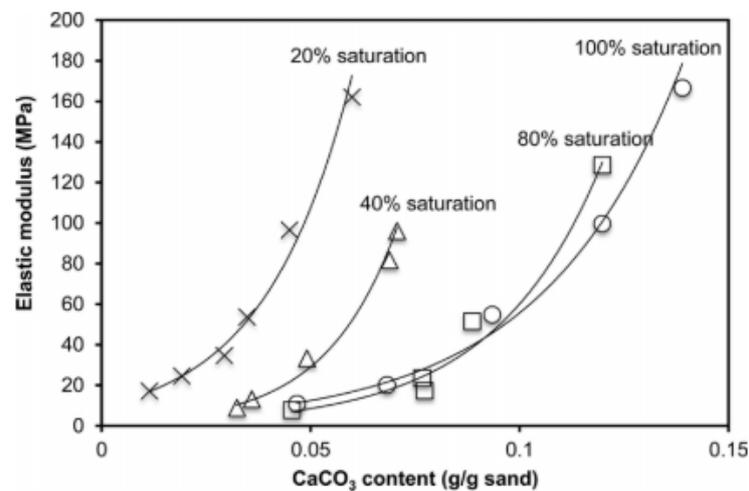
Figure 14: Variation of stiffness with CaCO<sub>3</sub> content and different saturation conditions for coarse sand (Cheng et al. 2013)
