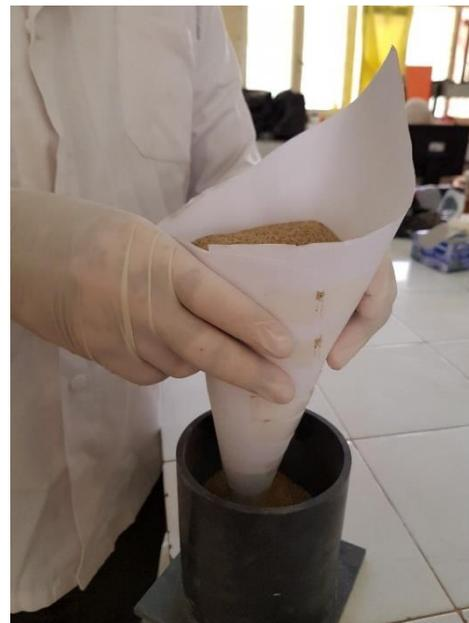
Figure 18: maximum voids ratio measurement
