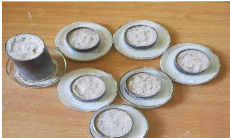
Figure 24: soil treatment by surface percolation method
