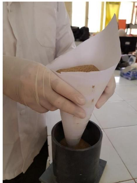
Figure 18: maximum voids ratio measurement
