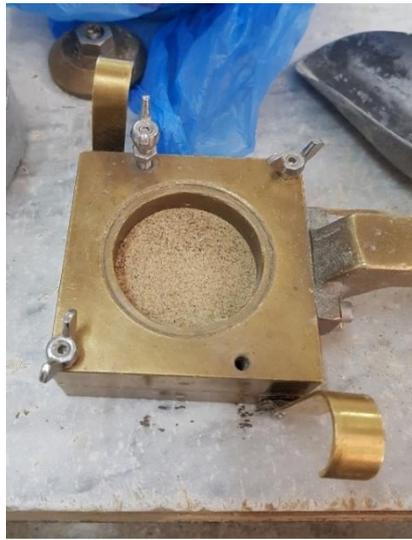
Figure 20: transfer sample into shear box
