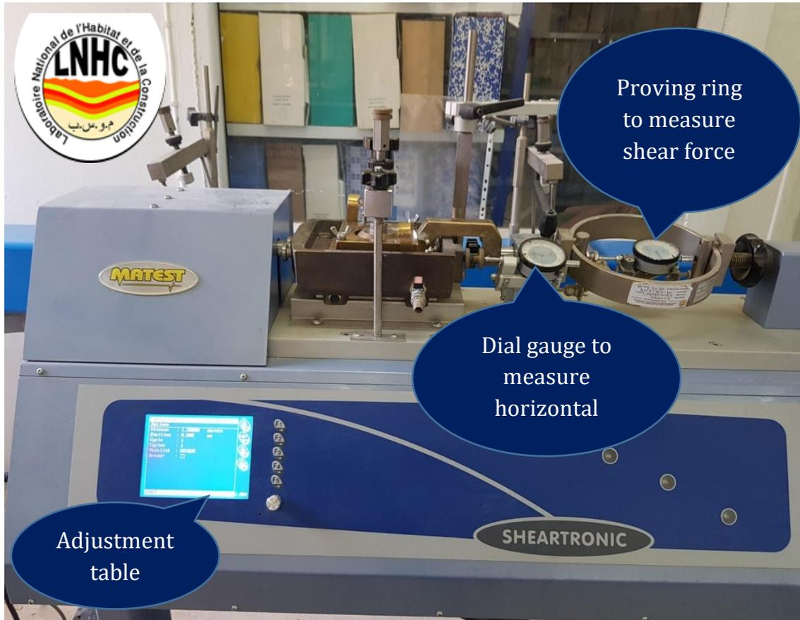
Figure 22: direct shear test instrument (LNHC-Batna)
