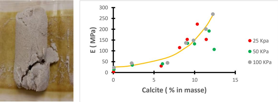
Figure 26: evolution of soil elastic modulus (data obtained from Dadda 2017)
