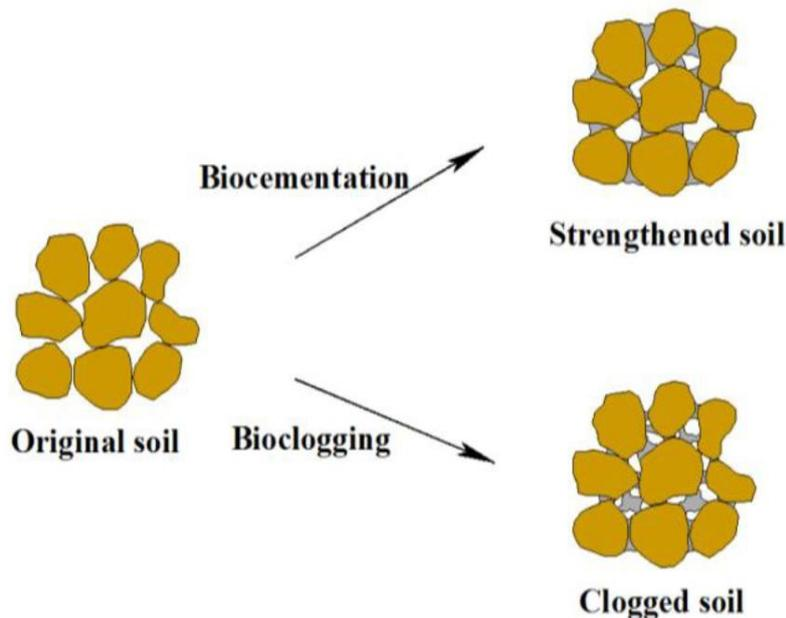
Figure 1: Schematic Illustration of bio cementation and bioclogging process by (Chu 2016)
