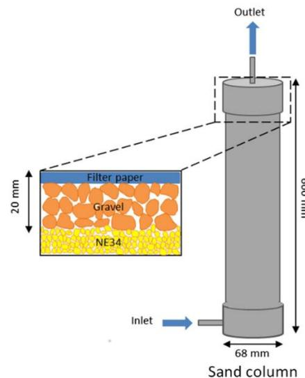
Figure 6: Injection protocol for biocementation process according to (Dadda et al.2017)
