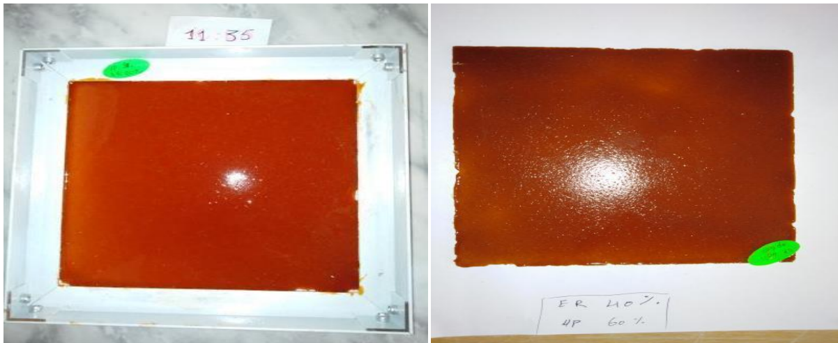
Figure 24: Le composite (UP/ER) moulée au contact.
