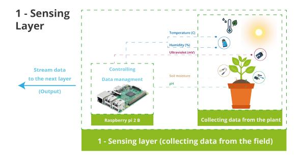
Figure 4.2: 1 - Sensing layer (collecting data from the field)
