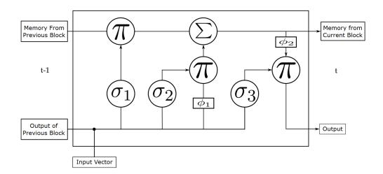
Figure 4.9: LSTM Repeating Module
