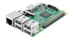
Figure 5.1: Raspberry Pi 2 model B
