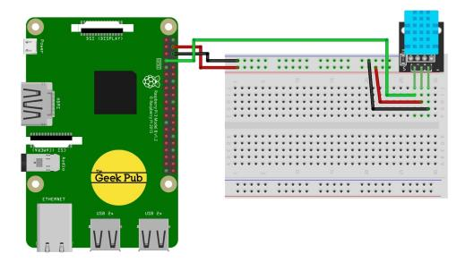
Figure 5.2: Raspberry Pi 2 connected to DHT11 sensor via the Breadboard
