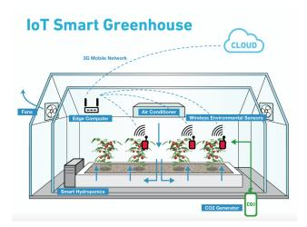
Figure 2.5: IoT in greenhouse (Smart Greenhouse)
