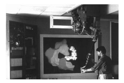
Figure 1-3: GROPE force feedback display (Mazuryk & Gervautz, 1996).
