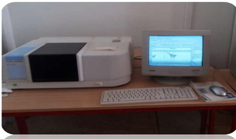
**Figure III.19 :** Appareil FT-IR.
