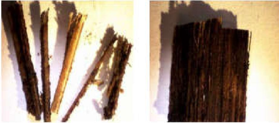
**Figure II.17 :** Fibres de tige du support dattier (grappe) [30].
