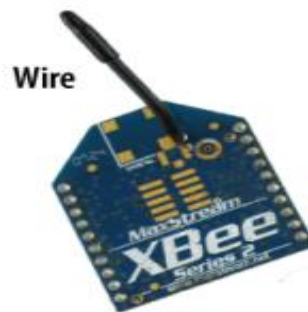
Figure II. 10 Whip or wire antenna [30]
