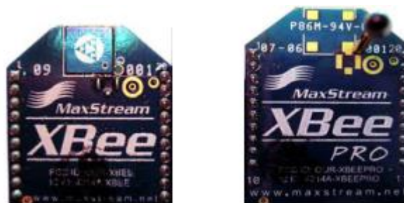
Figure II. 8 XBee-STD with chip antenna and XBee-PRO with whip
