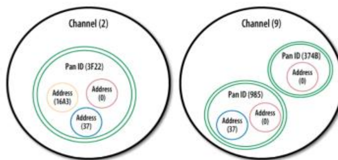
Figure II. 21 Venn diagram showing channel, PAN and addressing
