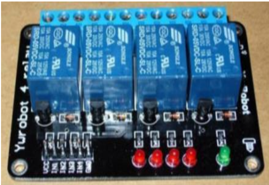
Figure II.37 : Modules de 4 relais (5V). [24]
