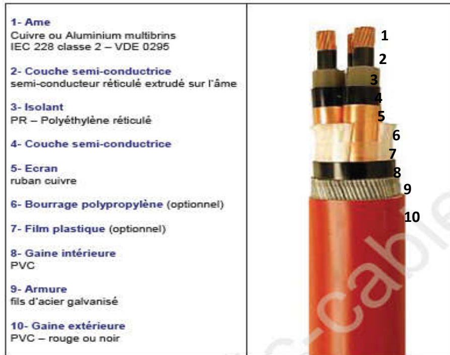
Figure 04: construction de câble XLPE. [7]
