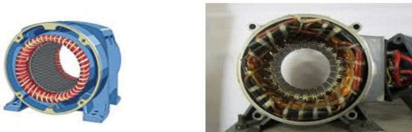
Figure (I.22) : Stator de la machine asynchrone
