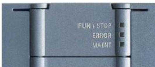
Figure III.20: LED dis-plays on the CPU
