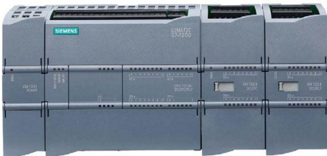
Figure III.18: S7-1200 station with CPU S7-1214, two SMs (right) and one CM (left)
