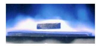
Figure 1.3 : A magnet floats above a superconductor
