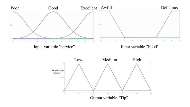
Figure 2.5 : Input and output variables membership functions.
