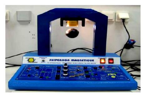
Figure 3.12 :Didastel magnetic suspension (Maglev unit)
