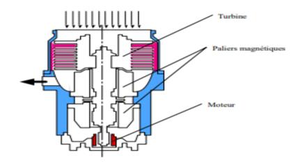
Figure 1.10 : Turbomolecular pump on magnetic suspension
