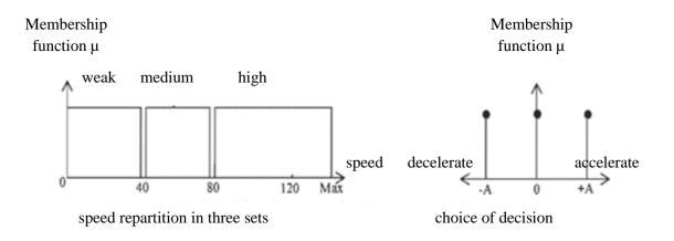
Figure 2.2 : Example of speed regulation with classic logic
