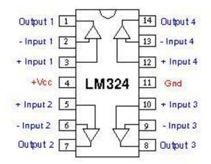
Figure 4.7: LM324 Pins connections
