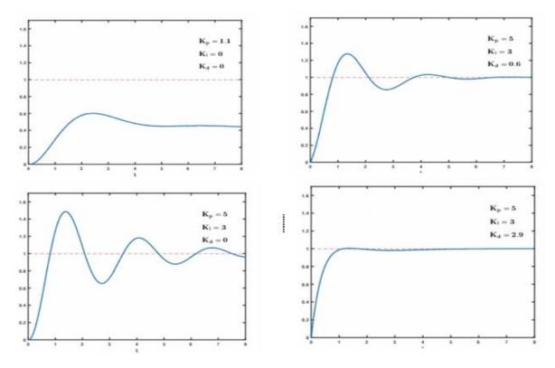
Figure 4.4: system output controlled by PID
