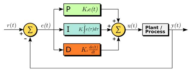
Figure 4.3 : A block diagram of a PID controller
