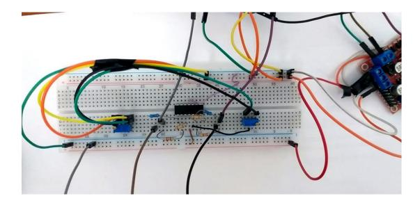
Figure 4.18: The realisation of OPAmp circuit
