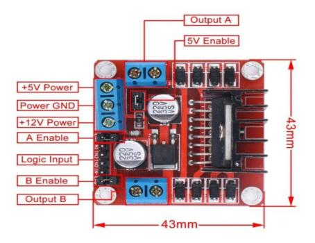
Figure 4.6: Board Dimension and Pins Function
