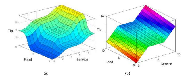
Figure 2.11: Decisions of a system based on : a) fuzzy system and b) classical logic
