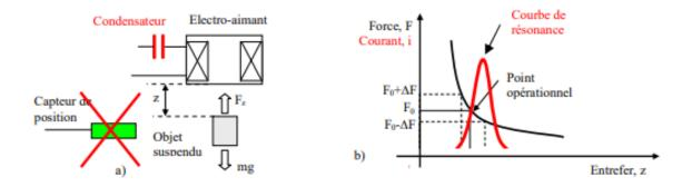
Figure 1.2 Principle of the resonant circuit electromagnetic suspension. a) Physical configuration b) Characteristic (Force-distance)
