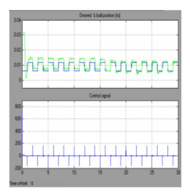
Figure 3.8 : Response of Fuzzy logic controller
