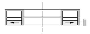
Figure 7 : Variable reluctance centering device
