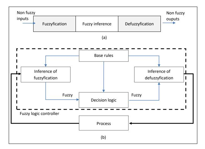
Figure 2.10 : Fuzzy logic controller : a) synoptic scheme b) principal parts
