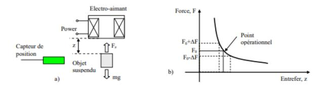
*Figure 1.1 : Principle of electromagnetic suspension a) Physical configuration b) Characteristic (Force-distance)*
