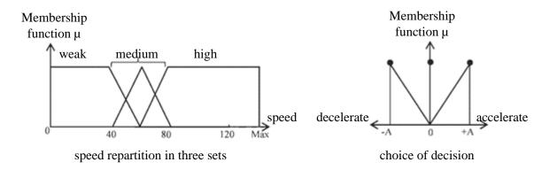
Figure 2.3 : Example of speed regulation with fuzzy logic.
