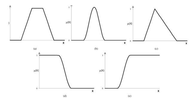
Figure 2.4 : Typical fuzzy set membership function shapes: (a) or trapezoidal, (b) Bell or Gaussian, (c) triangular, (d) Z-shape and (e) S-shape
