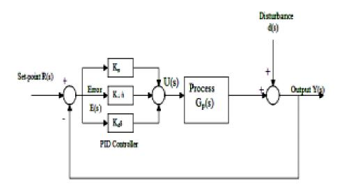
Figure 3.13 : Schematic of conventional PID Controller
