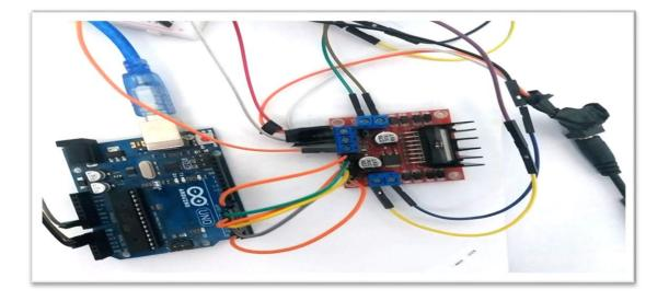
Figure 4.14 : L298N and arduino circuit
