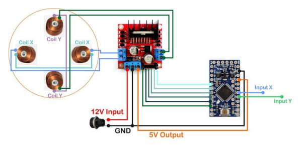
Figure 4.13 : L298N and arduino circuit
