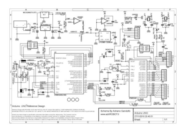
Figure 4.5: Circuit diagram of Arduino Uno
