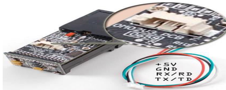
Fig. IV.7. Fingerprint sensor module hardware interfacing.
