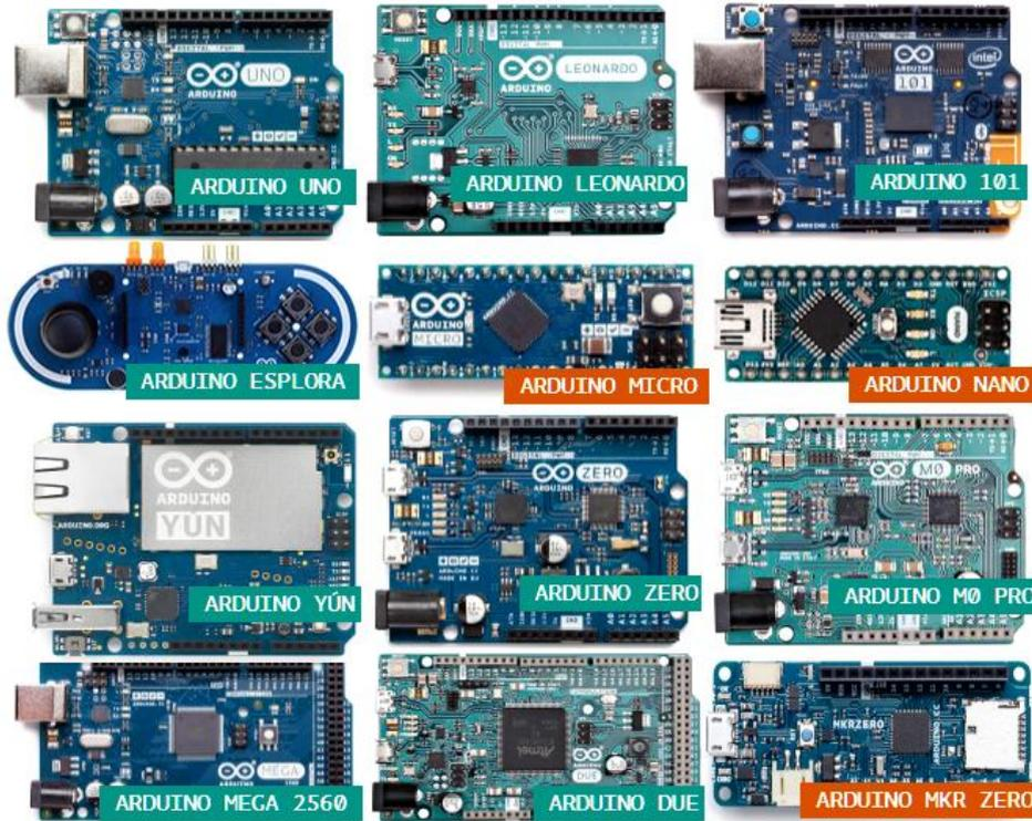
**Figure II.1.**The different Arduino boards [13].
