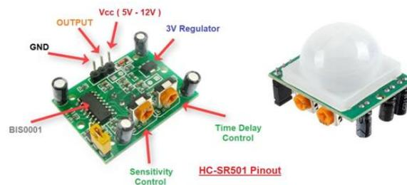
Figure II.6. PIR sensor [29]
