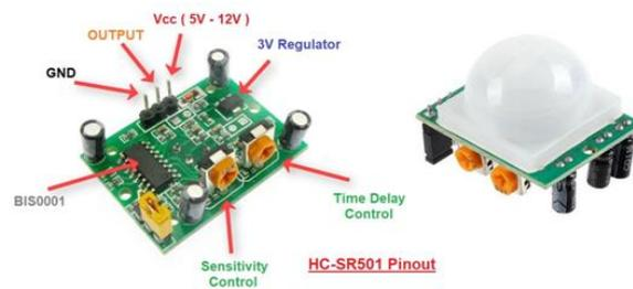
Figure II.6. PIR sensor [29]
