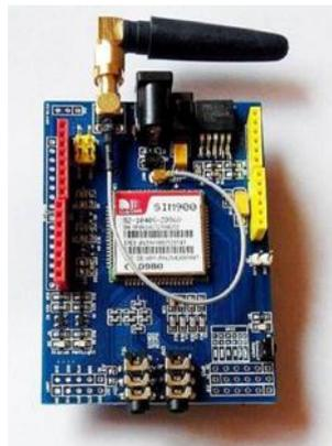
Figure II.9. GSM MODULE [33]
