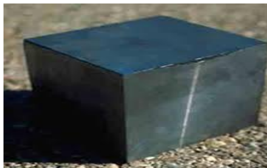
Figure I.5 : Lingot de silicium.
