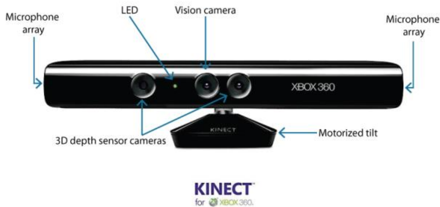
Figure 3.3: the depth sensors of camera Kinect.
