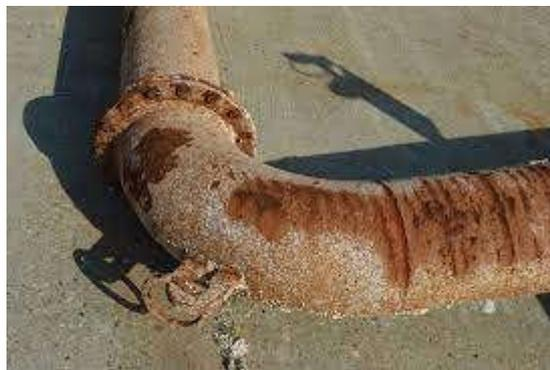
**Figure(I.1):** la corrosion uniforme
