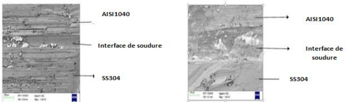
Figure. II. 17. Microstructure du joint soudé[3].
