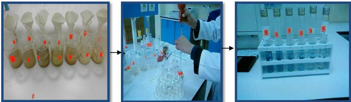
**Figure 2.9.** Le dosage de phosphore assimilable
