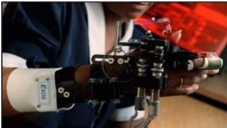
Figure 1.10: EXOS data gloves produced by NASA in the 1990s had very intricate external sensors to detect finger movements with high precision.
