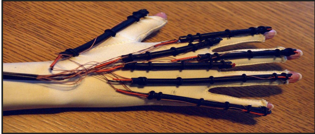
Figure 1.5: The first wired dataglove [3].
