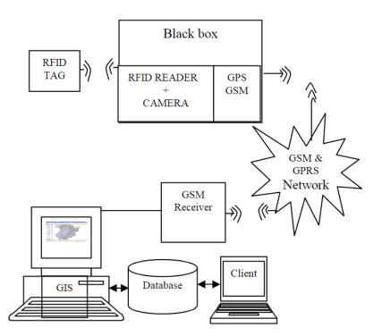
Figure II.1: Architecture of waste monitoring system
