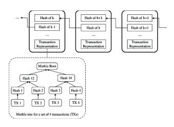
Figure 1.7: Illustration of a chain of blocks where transactions in a single block are represented by a merkle tree
