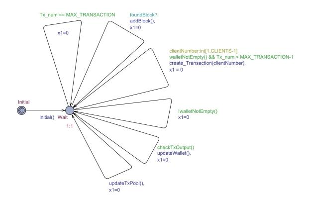
Figure 3.3: Automata of the client
