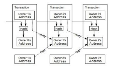
Figure 2.5: Transaction linking
