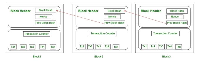
Figure 2.1: Block linking
