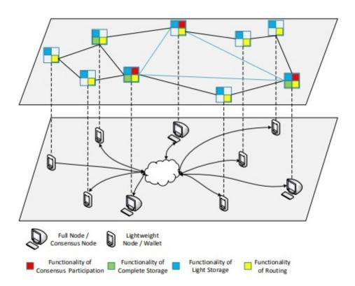
Figure 1.4: Illustration of roles of nodes in a permissionless blockchain network with P2P links between consensus nodes shown in blue
