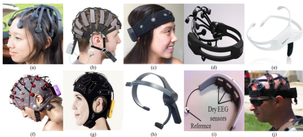
Figure 2.5: Diverse wireless portable headsets and acquisition methods for EEG recording. (a–c) Miniature Wireless Acquisition Systems by Cognionics with the Quick-20 Dry EEG Headset, 72-Channel Dry EEG Headset, and Multiposition Dry EEG Headband, respectively; (d and e) EPOC and Insight wireless EEG acquisition systems by Emotiv; (f) g.Nautilus wireless EEG acquisition system by g.tec; (g) ENO-BIO 8 wireless EEG system by Neuroelectrics; (h) MindWave Double-column image proportions.
