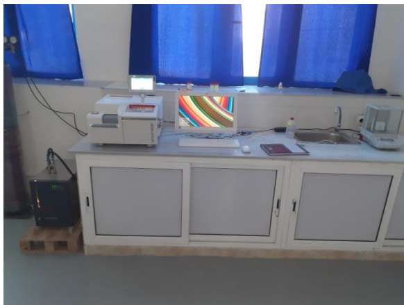
Figure.II.4. Differential Thermal Analysis (DTA) / Thermogravimetric Analysis (TG) Device
