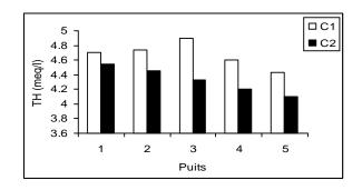
**Figure 5**: Space variation of the values of total hardness on the level of C1 and C2.
