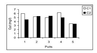
Figure 7: Space variation of the values of the Oxygen dissolved on the level of C1 and C2
