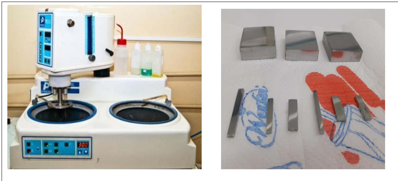
Fig.II.3. A mechanical polisher and samples after polishing.
