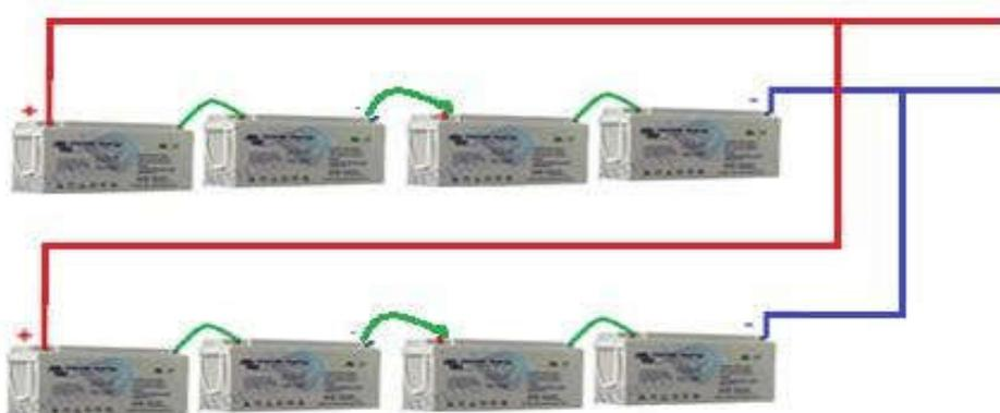
Figure .2-4 raccordement des batteries
