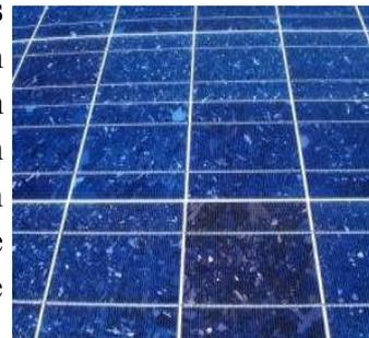
Figure 1-17 cellule poly cristalline
