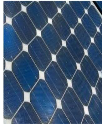
Figure 1-16 cellule mono cristalline
