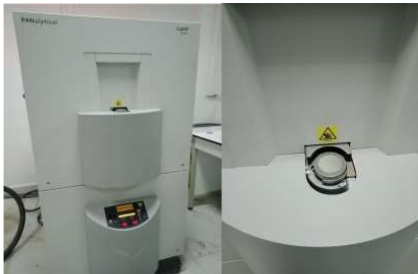
Figure III.2 : La diffraction des rayons X (DRX)
