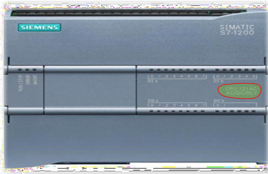
Figure III. 4 : La CPU S7-1214C (AC/DC/RLY).
