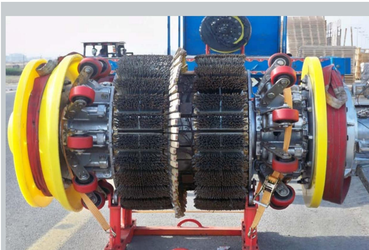
Figure III.3. L'outil d'inspection Magnetic Flux Leakage (MFL)
