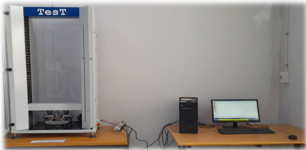
Figure.III.3. Machine universelle de type TesT.GmbH.112.5KN.2017
